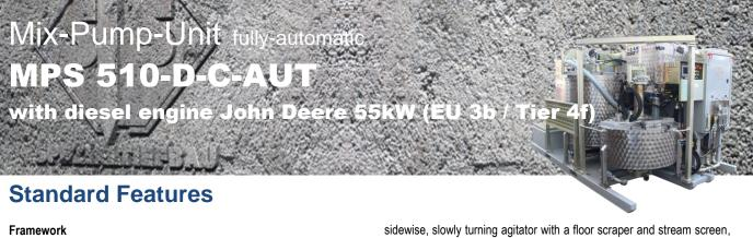
skid steel frame, partially enclosed and with partition panel, floor and oil pan, central towing device, lashing points for truck load securing, fork lift guides crosswise, machine room sound proofed, lockable doors, finishing 2K-paint RAL 5005 (signal blue) or on customer desire unicoloured
