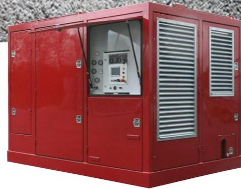
The achievable max. pressure and max. flow rate depend on plunger diameter, medium and the installed drive power.
