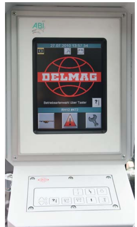
Control panel of DELMAG drill rig with keypad and big touch screen
