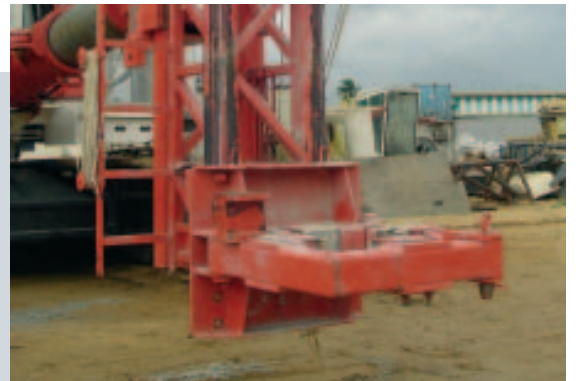
Pile Gate attached to a Fixed Lead.
