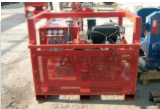
Hydraulic Power Pack.
