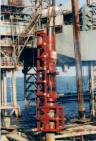
EU-Type Lead for pipe piles with striker plate for piles up to 1.500 mm of diameter.
