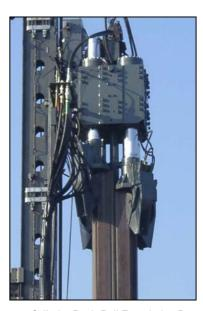
4 Cylinder Push-Pull Foundation Box Pile on Liebherr LRB255 - UK
