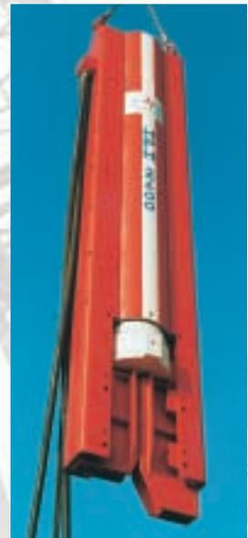
In the case of the HPH2400 and HPH6500 special off-set leg inserts can be supplied to drive larger pairs of sheet piles.
