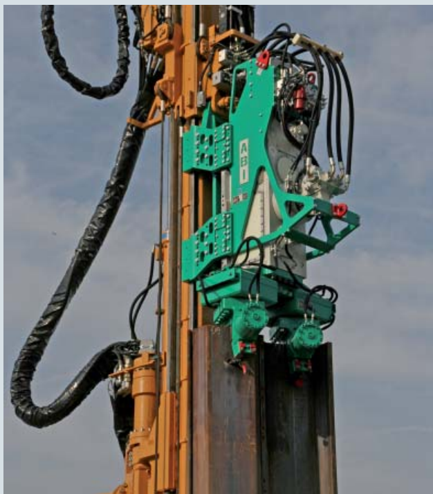
Variable moment vibrator MRZV-VV with double clamp assembly for driving double U- and Z-shaped steel piles and casings
