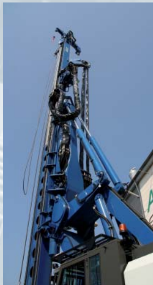
SD-kinematics of fixed leader mast
