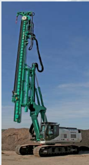
HD-kinematics of telescopic leader mast
