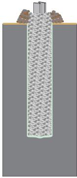
The finished pile. For higher bearing capacity the fresh pile can be reinforced.
