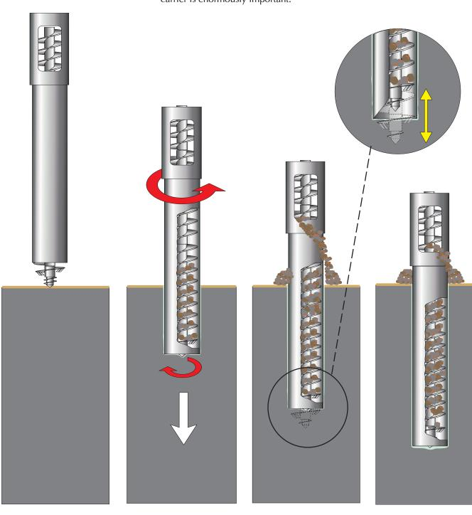
Vertical aligning of auger and casing.
