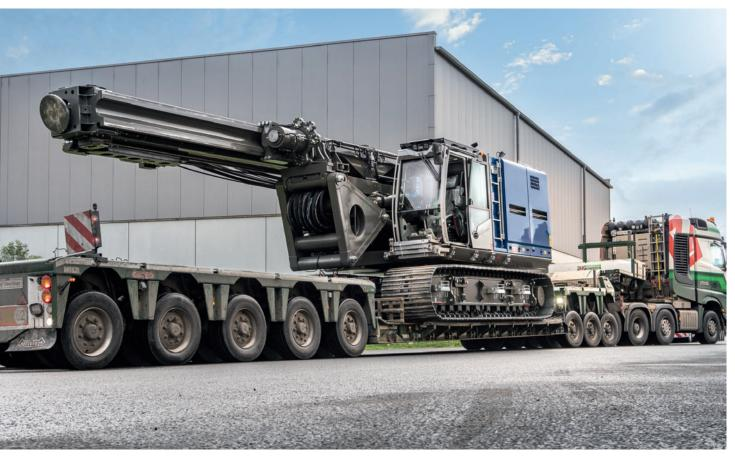
Transport situation with counterweights and base plate removed. The transport weight can also be reduced further by removing the track units.
