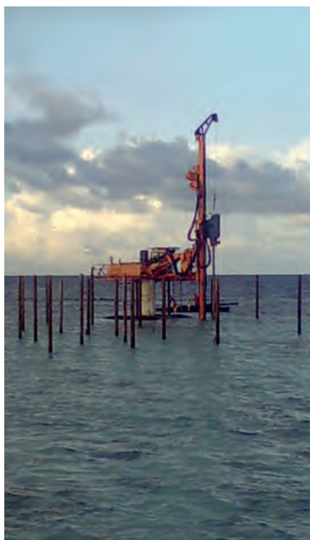
ABI groyne piling machine - between the crawler and upper carriage an intermediate piece (pylon) is mounted, so that the machine can be used for pile driving in shallow waters.
