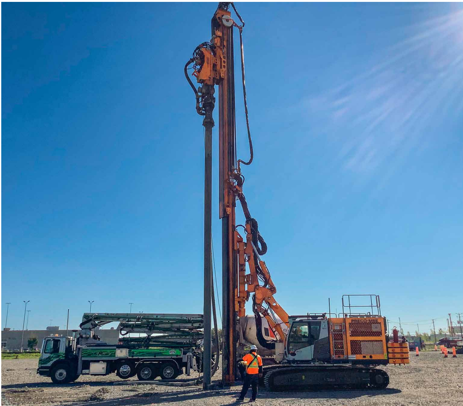
Photo: ABI MOBILRAM TM 20 with vibrator MRZV 20VV
