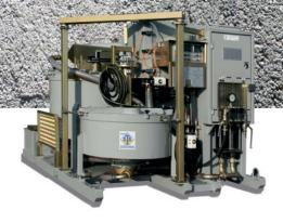
pumping down automatically controlled, screw conveyor automatically controlled, all butterfly valves are pneumatically controlled
