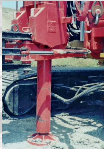
Mast foot cylinder and hydraulic auger guide
