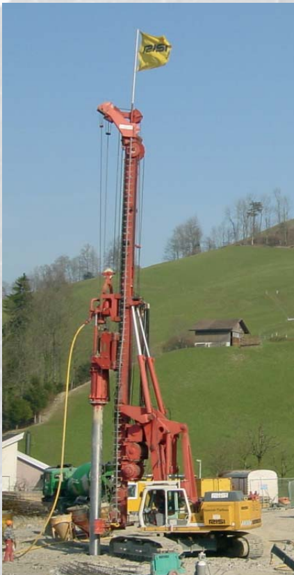
Drilling with dual rotary head (DDK)
