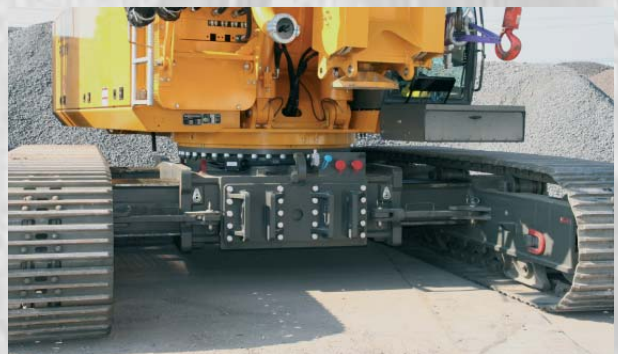
Telescopic undercarriage with connections for a casing oscillator
