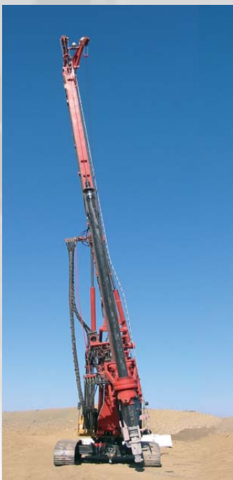
Lateral inclination of leader mast
