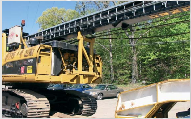
Transport without counter weight, with transport support for the leader mast
