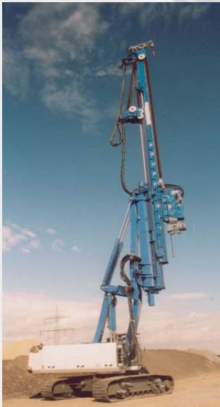
Kinematics of ABI MOBILRAM-System TM 20/25 with two folding down cylinders
