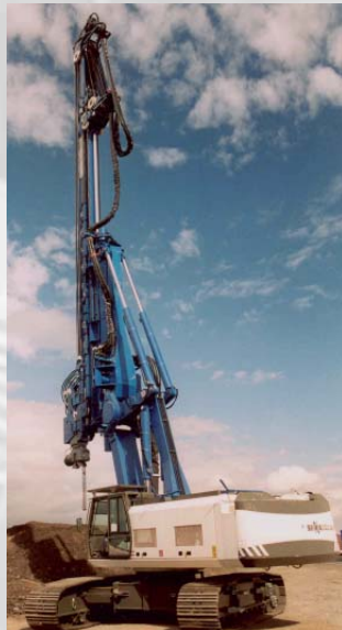
Kinematics of ABI MOBILRAM-System TM 20/25 with two folding down cylinders
