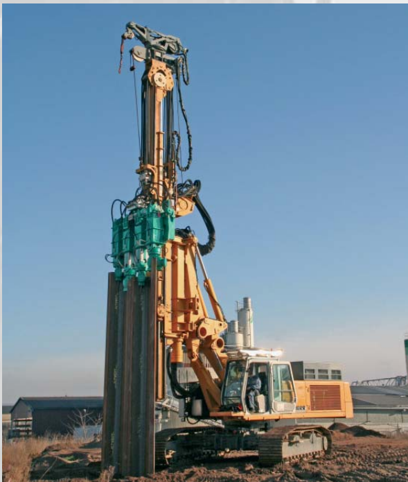
Universal press HPZ 500-720 with adjustable section width
