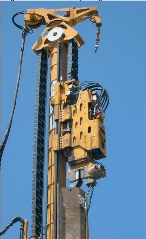
MRZV-V with dual Z-shaped sheet piles
