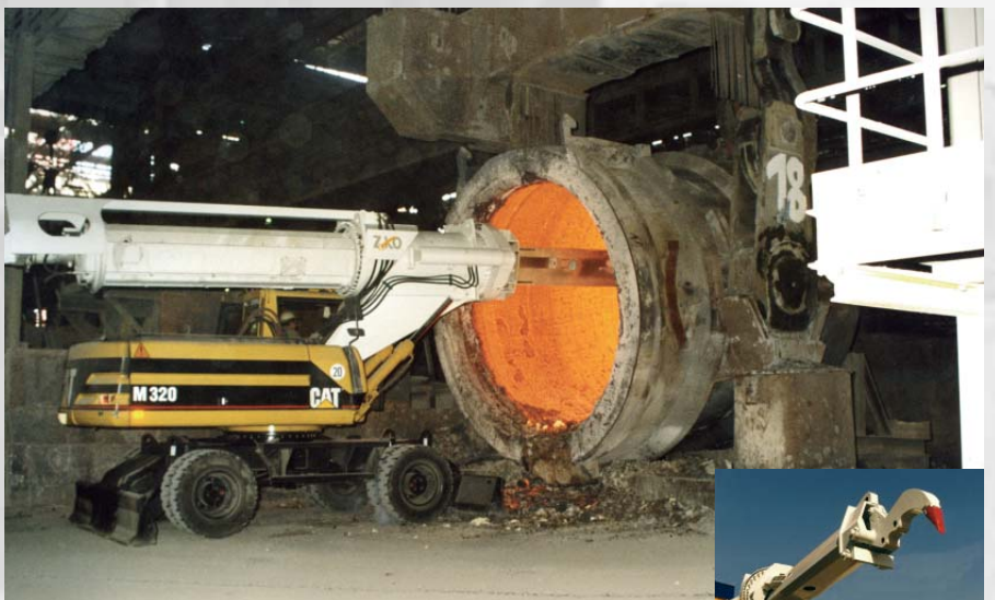
Special furnace cleaner on CAT carrier
