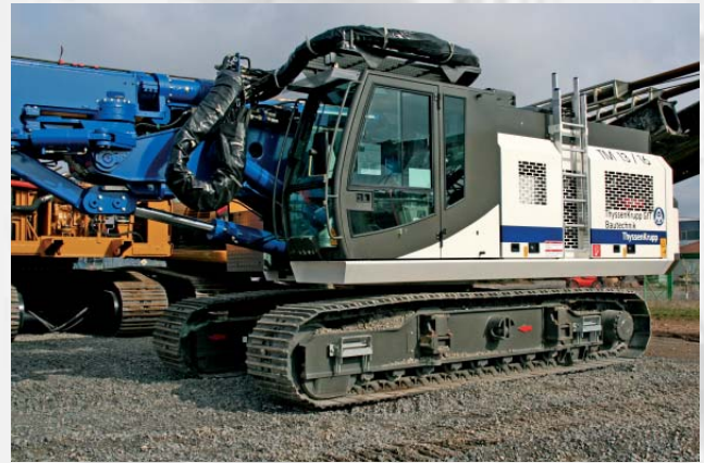
Carrier SR 35 with telescopic undercarriage and detachable counterweight
