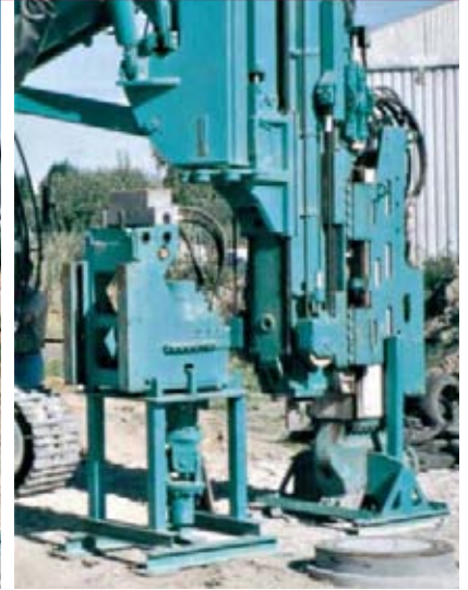
The docking system allows swapping of attachments within 5 minutes
