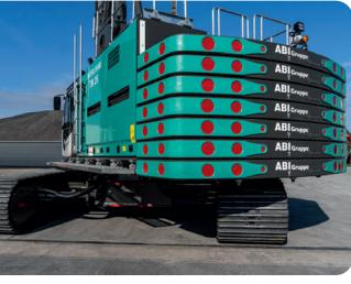
The stackable counterweights can be removed for transport.
