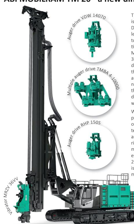
The new ABI MOBILRAM TM 26 is equipped as standard with the Docking-System D6, which enables various working attachments to be changed quickly and effectively. These include, for example, MRZV-VV vibrators in the sizes 30VV and 36VV, the VDW 14070 double auger head system or the ABI Quadmix TMBA 4-10000 auger drive. Due to the large number of working attachments, the TM 26 covers a wide range of different special civil engineering works.
