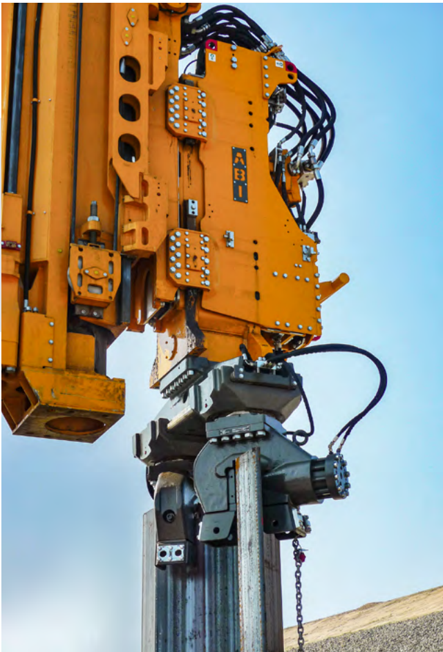
With a double clamp assembly MZK the force can be transferred optimally to double steel sheet piles or pipes.
